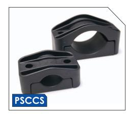
The Single Hole type cable clamps fasten a wide range of single and multi conductor low and high voltage cables. Designed to provide superior mechanical strength, ideal for installations where cables are subject to short circuits. The wide contact area provides a controlled pressure on the cable and prevent damage to the conductor insulation.
